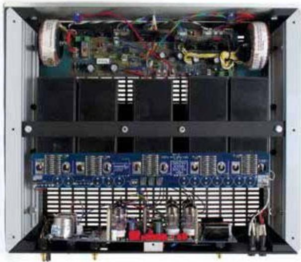
Interior of NAT, fully dual mono and with a battery of voltage power 6N23P-EV
